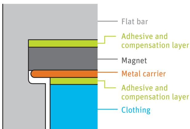
Fig. 3: Details of EasyTop
