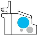
The cylinder roller is the key to every carding machine. Cylinder clothing takes over the fibers from the licker-in and is responsible for the main carding action with the flexible flats.
