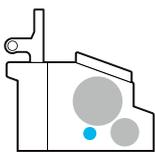
The licker-in wires are responsible for opening the fiber batt in the revolving flat card and transferring the opened fibers to the cylinder. Trash is removed at the licker-in. A gentle and even opening of the fibers at the licker-in is essential for the card sliver and yarn quality.
