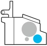
The doffer wire takes over the fibers from the cylinder. The transfer ratio and the uniform transfer of the fibers are important for achieving an optimal carding result. The quality of the doffer wire, in conjunction with precise settings, determines the smooth function of the fiber take-up from the cylinder to the doffer.
